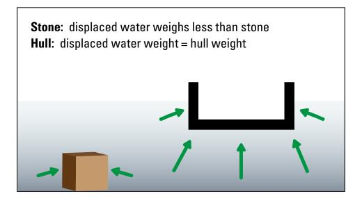
In my theory, the barges used for stone transport are not wooden planks roped together with a flat top surface. Instead, the barges were built from wood, similar to an open rectangular box, with a specific depth and flat bottom for better stability on the water. All barges were built to meet certain specifications, keeping the sluices' dimensions to a minimum.
