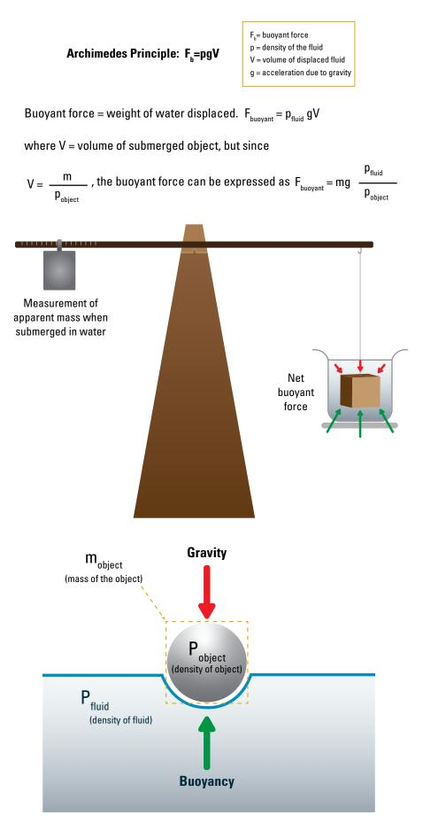
Buoyancy, or thrust (upthrust), is an upward force exerted by fluid on an object fully or partially immersed. Pressure increases with depth due to the weight of the overlying fluid.
