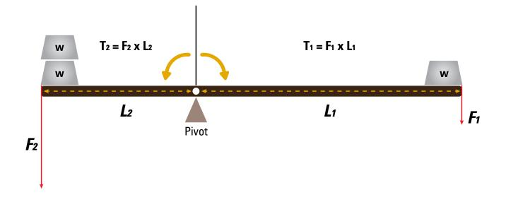
In equilibrium (balance)  $T_1 = T_2$  $F_1 \times L_1 = F_2 \times L_2$
